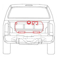
12 x 60 - 12 x 48 Under Tool Box In Bed Fuel Tank (Short Bed) - 38 USG 12 x 12 x 60 Under Tool Box In Bed Fuel Tank (Long Bed) - 42 USG
