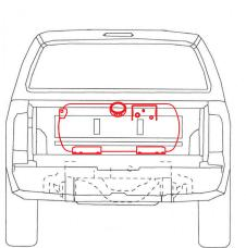
12 x 60 - 12 x 48 Under Tool Box In Bed Fuel Tank (Short Bed) - 38 USG 12 x 12 x 60 Under Tool Box In Bed Fuel Tank (Long Bed) - 42 USG
