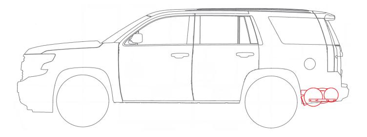
10 x 35-13 x 33 Under Vehicle Fuel Tank - 22 USG
